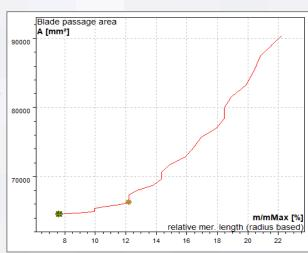
Blade passage: 64567 mm<sup>2</sup> Distance B2B: 280.1 mm Max. sphere radius: 78.189 mm Distance H2S: 213.2 mm
